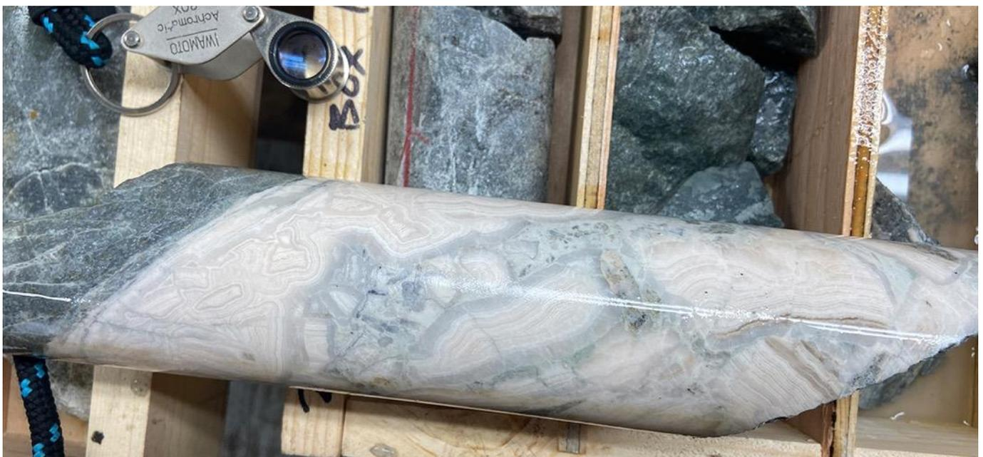
Figure 8 drill core (HQ) interval 212.35 – 212.50m hole 20AU09. Example of a brecciated colloform quartz vein “dilational zone”.
