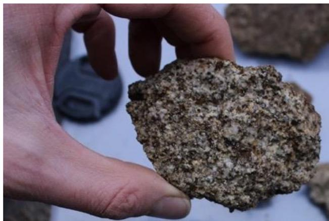
Figure 5 Quartz-feldspar-biotite granite samples from road cut 20AT001T. Sample 707517 (left) assay returned 1.63g/t Au from 66-67m and includes 1-6mm wide quartz veins (sheeted vein sets). Sample 7075529 (right) assay returned 1.89g/t Au 78-79m.
