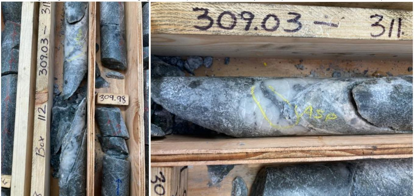
Figure 7 Example of a quartz-sulphide vein “dilational zone” intersected in hole 20AU08. The photo on the left is an interval of NQ drill core from 309.18 - 309.78m. The photo on the right is a zoom in on the interval 309.18 - 309.38m with an arsenopyrite vein cross cutting a quartz vein highlighted with yellow markings.
