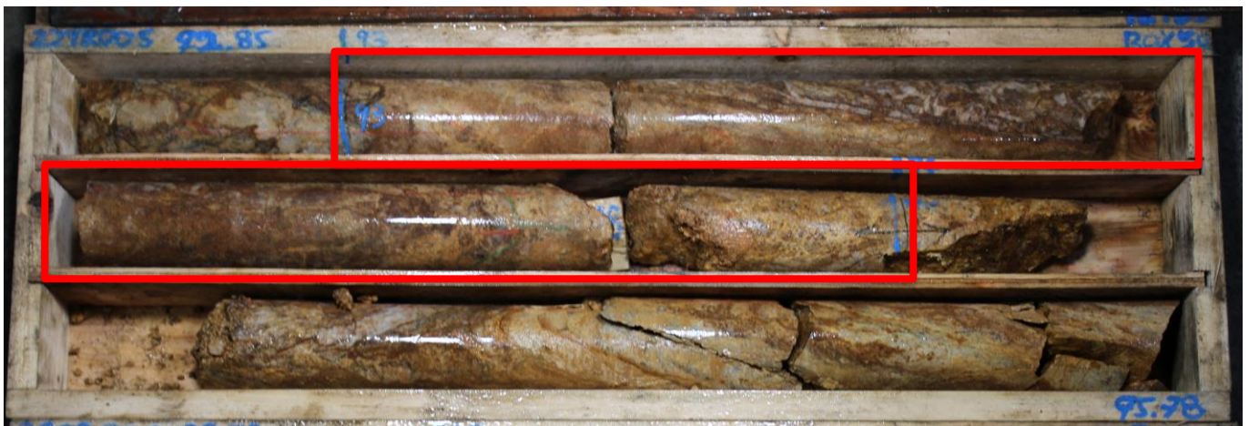
Drill hole 22TR005 with 1.0m @ 6.7g/t Au from 93m (red boxes). Intensely brecciated, yellow-brown granite gneiss with common high angle, pink to grey quartz/limonite/tourmaline veins (high-angle, antithetic veins).
