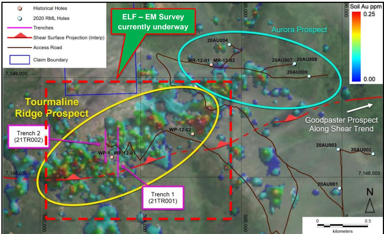
Figure 4. Anomalous surface geochemistry extending over a 1.8km x 750m area with a prospective ENE-SSW trending shear extending along strike from the Goodpaster Prospect to the northeast. Section line Trench 1 & 2 is reference for Figure 3. (RML ASX Announcement 26/11/2019).
