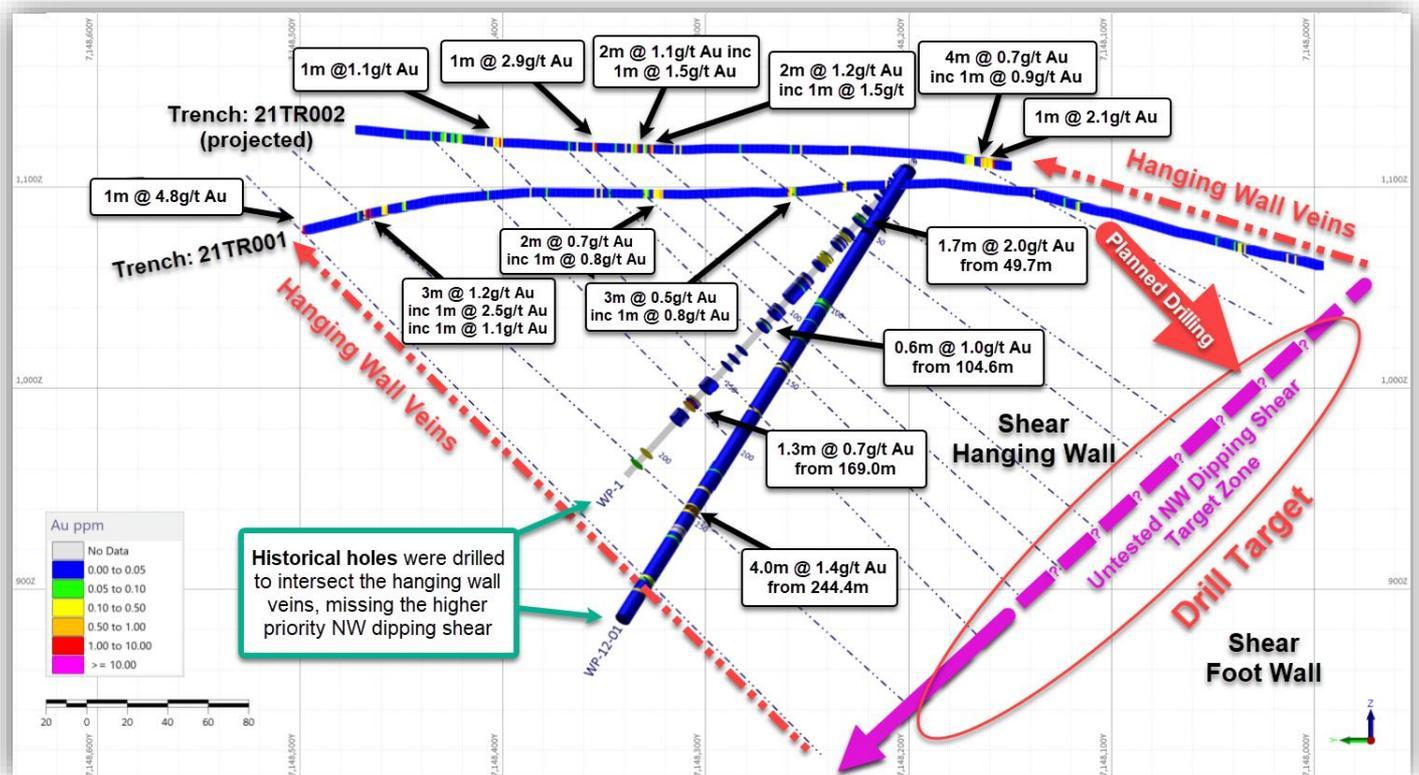
Figure 3 Tourmaline Ridge Prospect cross section including full assay results on trench 21TR001 and 21TR002. Historical holes WP12-01 and WP-1 are included, aiding interpretation of antithetic hanging wall veins relative to an interpreted northwest dipping shear, prospective for Pogo-style mineralisation. See section line reference on Figure 4 (Trench One and Trench Two).
