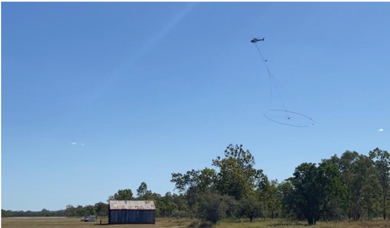
Figure 3 VTEM geophysics survey flight underway at the Wollongorang Project 2021.
